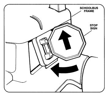
**3.** If the stop sign should ever come unattached from the schoolbus frame, snap back into place by pushing the top up and in and then pulling bottom down and in as shown.
