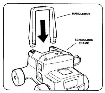
Snap the walker handlebar onto the schoolbus frame as shown. The handlebar will fit correctly either way; there is no front or back.
