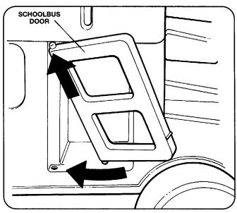
If the schoolbus door should ever come unattached from the schoolbus frame, snap back into place by placing the top peg in top hole and then sliding the bottom peg into bottom hole at an angle as shown.
