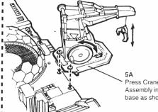
Press Crane Assembly into the base as shown.
